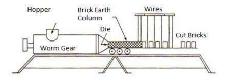
Figure 2.5 Worm Gear Type Machine Moulding
