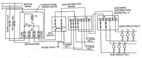
Typical House-Wiring Circuit
