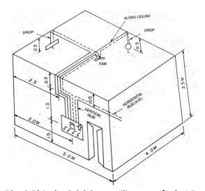
From SB to fan =1.5(VR) + 0.5(HR) + 0.5(rise) + 2.0 (along ceiling upto fan)=4.5mts From SB to lamp=(1.5+0.5+0.5+4+0.5)mts=7 mts From SB to tube point=(1.5+0.5+0.5+2+2.5+0.5)mts=7.5 mts From point of entry of circuit into room upto SB= 2(HR)+1.5(VR)=3.5 mts
