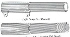
(Heavy Gauge Screwed Steel Conduit With Coupler Fig. 3.11
