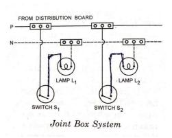
• In joint box system, the connection to electrical points are given through joint made in joint boxes by means of suitable connectors or joint cut-out.
