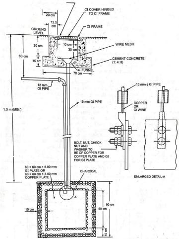
Note-Three or four buckets of water to be poured into sump every few days to keep the soil surrounding the earth pipe permanently moist.
