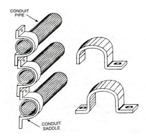
> Saddle are used for fixing the conduit where clips cannot provide a firm enough hold or a single screw cannot be dependent upon for fixing.
