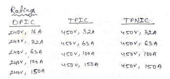
> Since no fuse is to be provided in neutral in DPIC switch fuses, where provision is made for fuses in both the wires, one fuse carrier is furnished with fuse elements and the other a thick copper wire.
